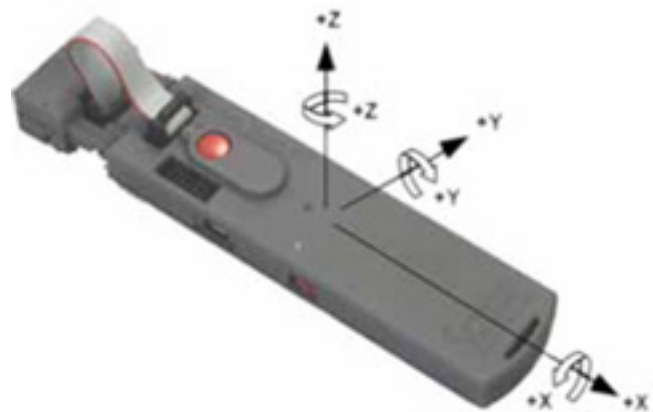
Figure 2. Enactive Torch (ET) and the orientation of the triaxial accelerometer. Taken from: https://github.com/CreativeRobotics/EnactiveTorchRT/blob/master/Instructions
